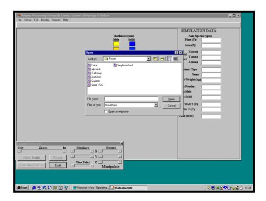
After the mould has been selected, it will appear on the screen. At this point the **Manipulate** controls can be used to rotate the mould to get check its shape. The X, Y and Z axes rotation bars are at the bottom right of the **Control Panel**. The orientation of the mould on the machine and screen are as shown below:
