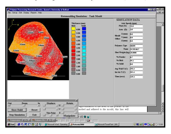
At any moment in time it is possible to call in the temperature rise graphs and information about the relative amounts of powder/melt/solid material. These will appear as Pop-up windows and can be positioned at any location on the screen, as shown below:
