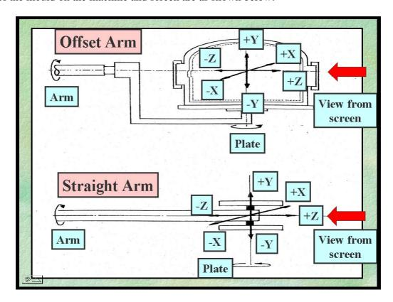
The orientation of the mould relative to the X, Y and Z axes can be altered as required using the **Position the Mold** heading under the **Set-Up** button.
