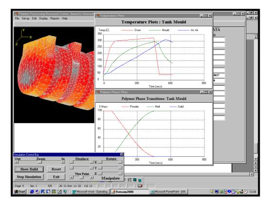
At the end of the trial the thickness at any point on the mould can be observed. This is illustrated below. A full summary of the trial and the results can be printed by selecting "Simulation Report" using the Reports button.
